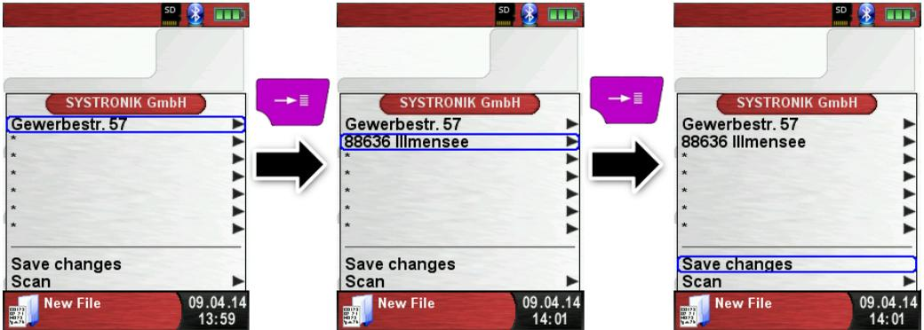
To delete customers in the database there mustn't be any measurements stored. Select the customer and choose „Scan“, if there are no measurements stored the request „Entry is empty delete?“ will occur. Confirm the request with “Yes“.
