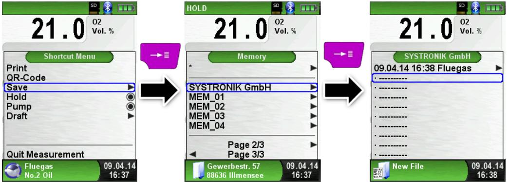
The file name and the storage location is shown in the lower bar. In this example: Storage folder: MEMORY/0000 and file name 0000\_01.txt:
