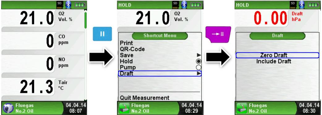
The measured draft is displayed continuously in the main display (red colored). After the confirmation of the draft value with “Include Draft” the value will be included in the record and will be displayed in black color.
