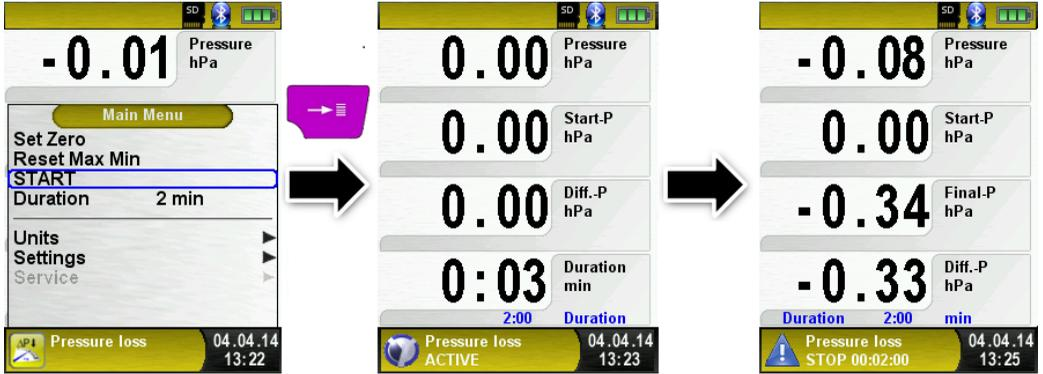
After the set elapsed time duration a signal sounds and in the information line the message "STOP pressure loss". The elapsed measurement time is also displayed. The readings are held in the main display, and you can then print the test report or save it to the MicroSD Card.
