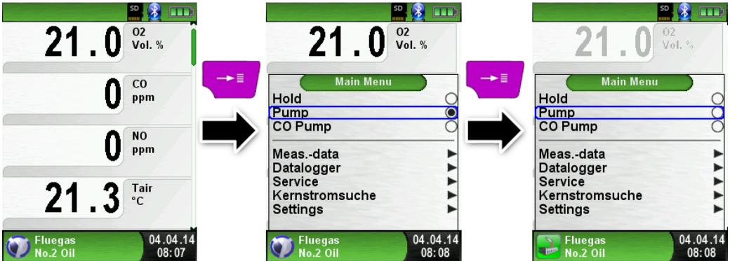
When the gas pump is switched off, the pump symbol is no longer shown in the status bar. Changes in the corresponding measured gas values cannot be ruled out, e.g. the O2 value may change as a result of lack of oxygen in the gas lines inside the device. If the gas pump remains off for a longer period of time, calibration in fresh air should be carried out before a new measurement is made.
