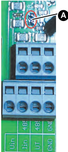
Fig. 12: Activating the terminating resistor
